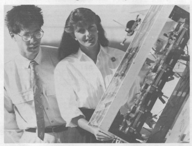
RECORD-SETTING EXPERIMENTAL MODULE is displayed by developers Clement Chiang (left) and Beth Richards (both 6221). The module includes a fluid cooling system for accurate temperature control and independent three-dimensional cell positioning capabilities. With these features and other Sandia-developed innovations, the module achieved an energy efficiency of 20.3 percent at standard test conditions of 25°C cell temperature and 800 watts per square meter of solar irradiance.
